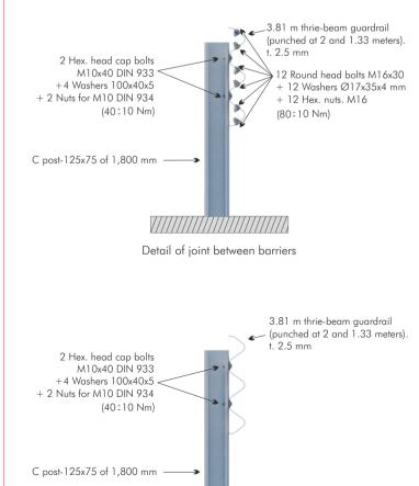
Detail of joint in intermediate post
