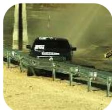
Essai : 4-11: Pick-up 2.270 kg - 100 km/h - 25°
