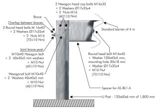
Detail of joint in intermediate post
